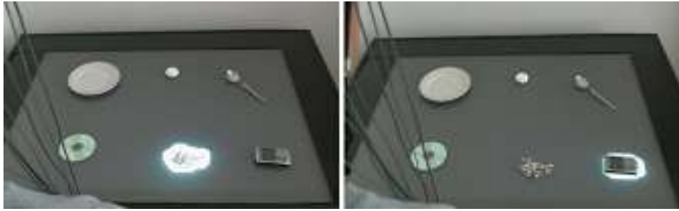
Figure 6. Multitouch display interface, where objects are enlightened one by one, triggering a P300 wave. Source: [137].
