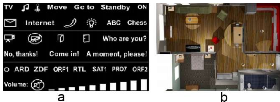
Figure 8. A (a) P300-based BCI for controlling (b) a virtual domotics environment. Source: [28].
