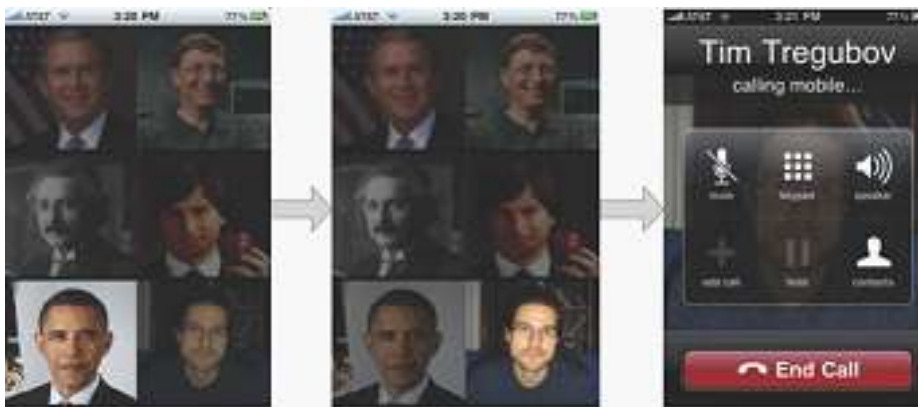
Figure 5. Contacts flash, one by one, detecting the user visual focus. A phone call is made to the chosen one. Source: [15].
