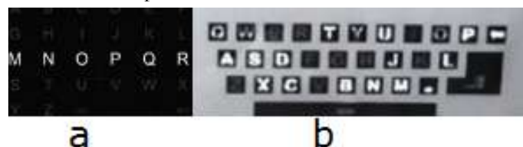
Figure 3. Spellers based on (a) P300 (b) SSVEP. Sources:[104],[51]
