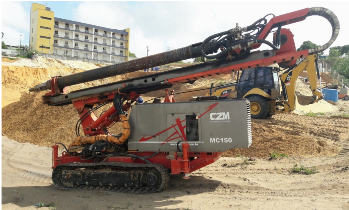
Figure 3.15 – MC150 drilling rig machine, manufactured by CZM.
