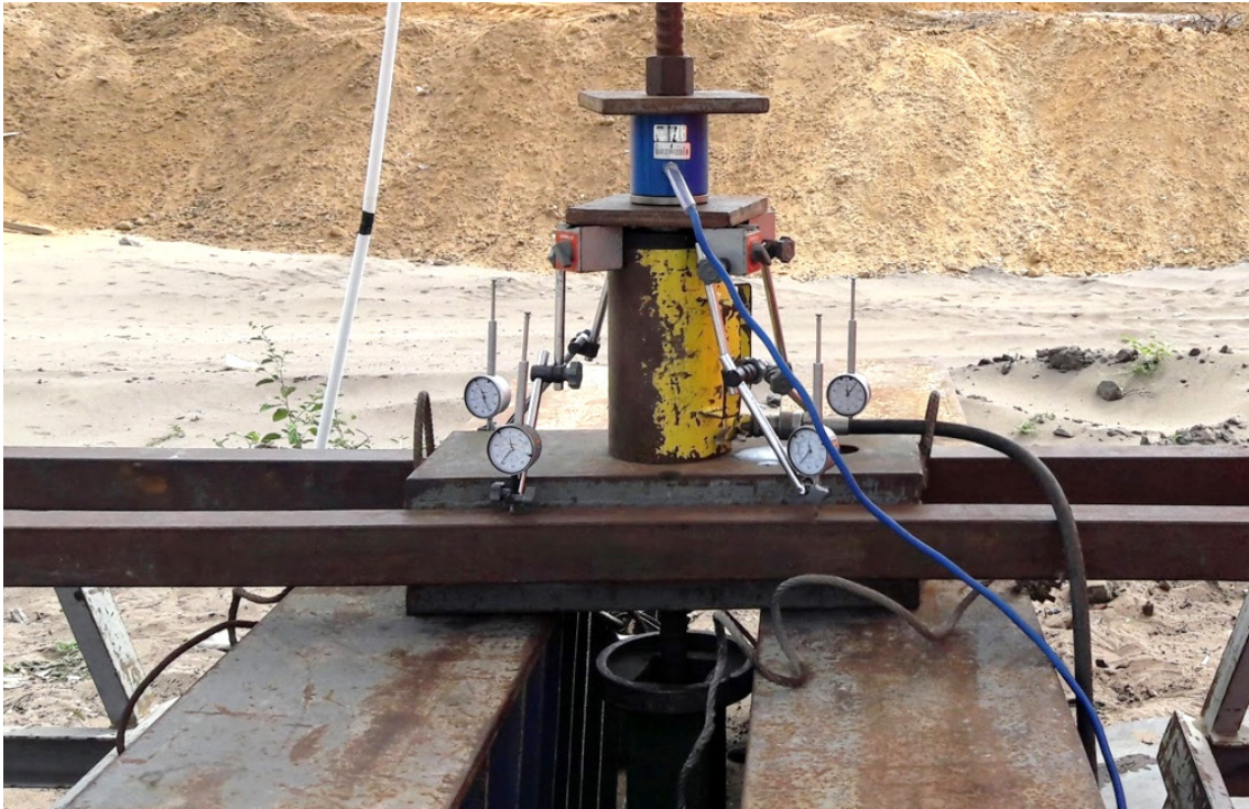
Figure 3.17 – Load test setup.
