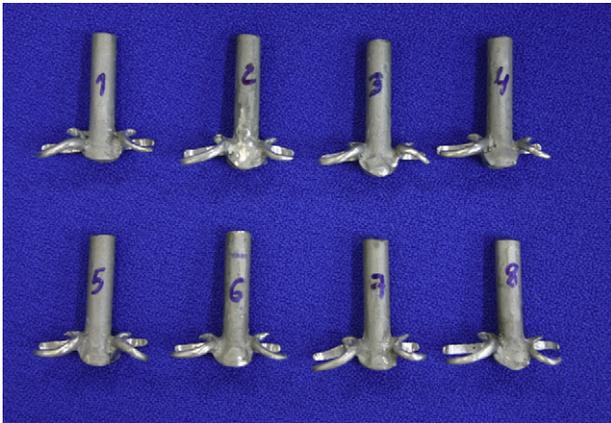
Fig. 2. View of specimens entirely made in Co–Cr.
