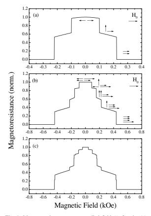
Fig. 1. Magnetoresistance versus applied field  $H_0$  for the (a) N = 3, (b) N = 5 and (c) N = 7 Fibonacci generations. The parameters are  $r \sim 0.33$  and a cubic anisotropy field  $H_{ca} = 0.5$  kOe.
