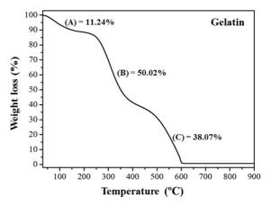
Figure 1. Thermogravimetric curve of natural gelatin.
