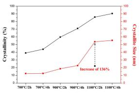
Figure 4. Effect of temperature and time of calcination on crystallinity and crystallite size.
