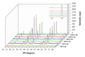
Figure 3. XRD patterns of MgAl<sub>2</sub>O<sub>4</sub> powders.
