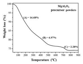
Figure 2. Thermogravimetric curve of MgAl<sub>2</sub>O<sub>4</sub> precursor powders.
