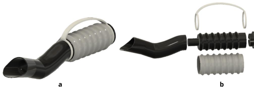
Fig. 6 3D adaptive eating device. (a) Final design. (b) Exploded view.
