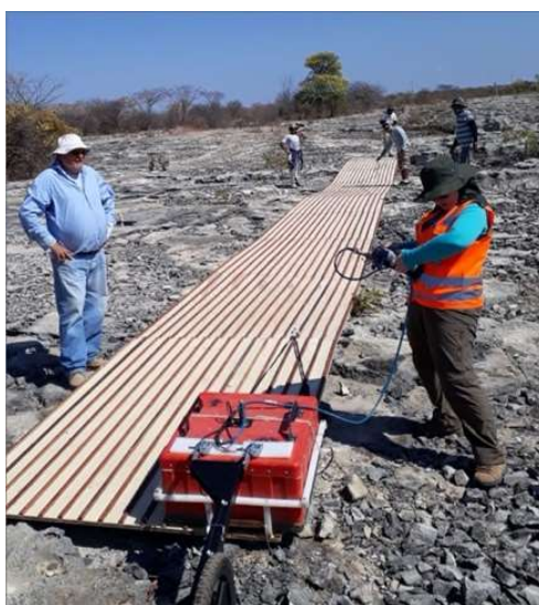
Figure 2: Photograph taken during the GPR survey in the AT area highlighting the use of wooden pallets. A 200 MHz GSSI antenna is mounted on wooden rails, which are fixed
