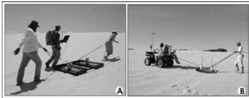
Figure 2: Data acquisition, using an antenna frequency of 100 MHz. The equipment was carried manually (A) and fixed to quadricycle (B) using antenna frequency of 200 MHz.
