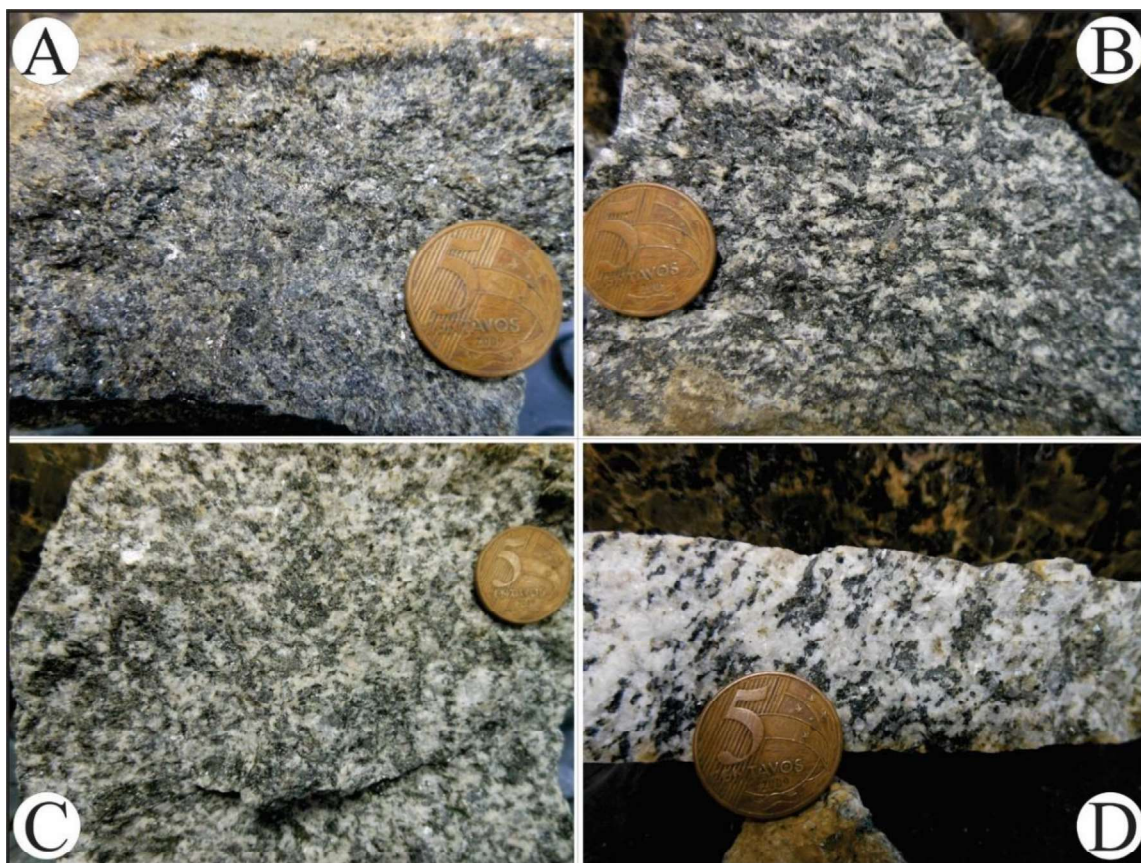
Figure 2. Typical macroscopic aspects of the São João do Sabugi pluton. A) Massive melanocratic rock (color index - CI~65%) typical of the gabbro-dioritic facies. Mafic minerals include pyroxenes and amphiboles; B) and C) Massive mesocratic rocks of monzodioritic facies, including more mafic (in B; CI~50%) and more felsic (in C; CI~35%) varieties. Amphibole ± biotite (± pyroxenes) are the main mafic minerals (black colors); D) Foliated leucocratic rock (CI~10) typical of the granodioritic facies (IC~10). Note preferred orientation ( S\gamma//S_3 ) of the mafic minerals (mainly biotite, in black colors).
