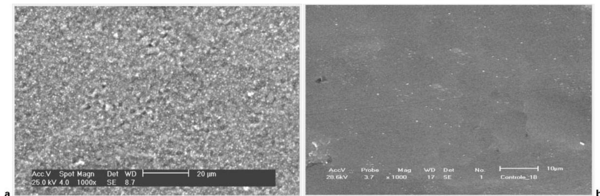
1 Both plasma *a* nitrided titanium and *b* control surfaces observed under SEM
