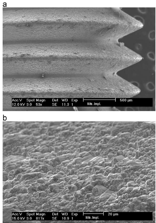
Fig. 6. (a) SEM image of the surface of the nitrided dental implant (150 Pa, 500 °C and 2 h) with its (b) detail.
