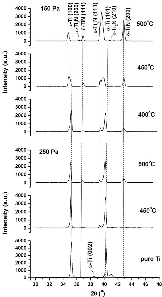
Fig. 2. X-ray diffraction spectra of pure Ti and the samples nitrided at pressures of 150 and 250 Pa, at temperatures of 400, 450 and 500 °C for 1 h.
