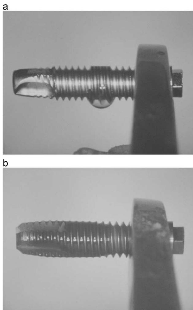
Fig. 7. Wettability test: the physiological serum drop coverage of the surface of (a) as-supplied and (b) nitrated dental implant after 60 s. Scale: dental implant screw is 4 mm in diameter and 9 mm long.
