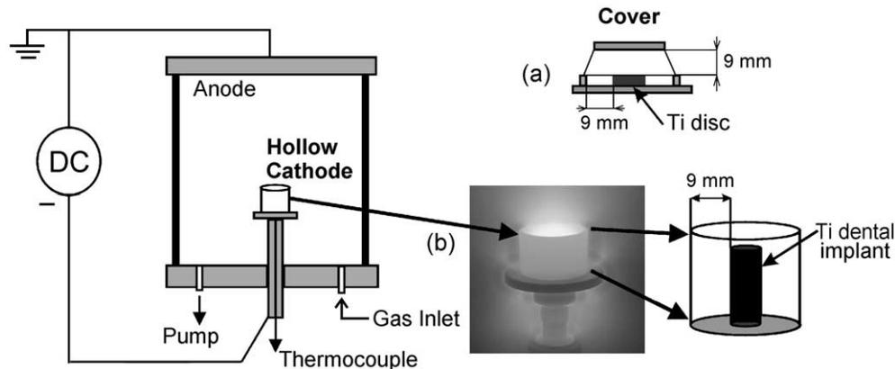
Fig. 1. The Hollow Cathode Discharge (HCD) nitriding system configuration with inserted (a) Ti disc and (b) dental implant.
