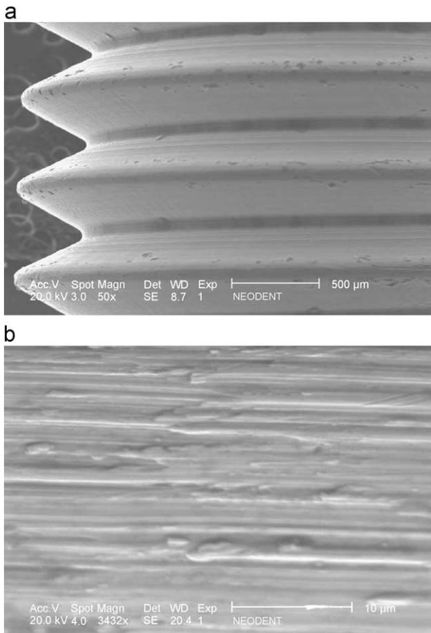
Fig. 5. (a) SEM image of the surface of the as-supplied dental implant with its (b) detail.
