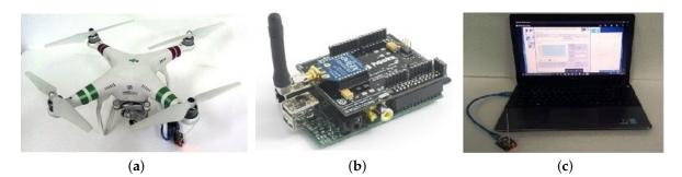
**Figure 7.** Hardware specification of the proposed multi-UAV system. (**a**) XBee module embedded in UAV Phantom 3 Standard; (**b**) XBee module connected to the power bank; (**c**) BS equipped with a XBee module.
