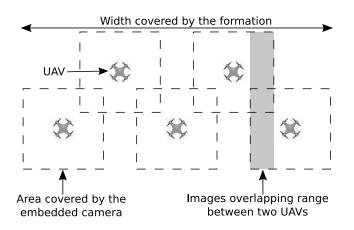
Figure 3. Flight formation for spiral scanning.
