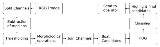
Figure 8. Sequence of steps of the proposed algorithm.
