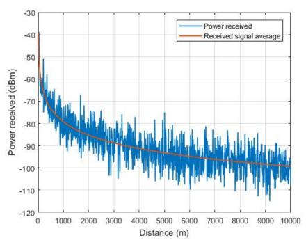
Figure 17. Simulated behavior of the power received by the XBee transceiver.
