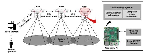
Figure 6. Architecture for the Multi-UAV system.
