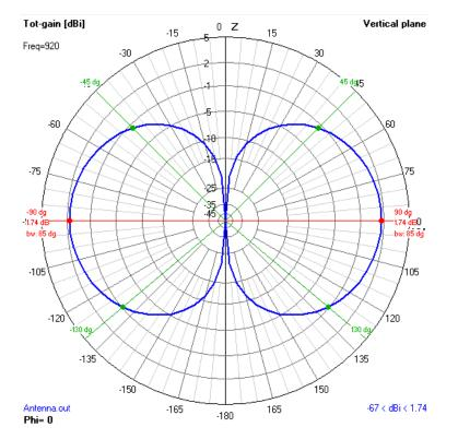
Figure 15. Analysis of the best position of XBee antenna by simulation using 4nec2 software.
