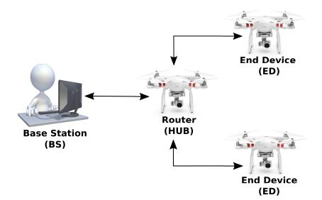
Figure 13. ZigBee devices in a scenario 1 with mesh configuration.
