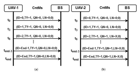
**Figure 9.** Flow of CntMs to the BS in a FANET: (**a**) UAV-1 completed the mission without detecting boats; (**b**) the imaging system located a boat, while informing the BS and preparing a DM.
