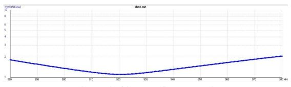
Figure 16. Simulation results of the operating frequency range of XBee antenna.
