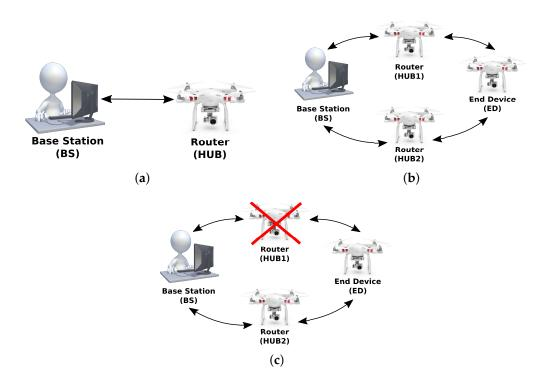
**Figure 14.** ZigBee devices in configuration scenario 2. (a) ZigBee devices in P2P configuration scenario; (b) ZigBee devices in a scenario without failure; (c) ZigBee devices in a scenario with failure.
