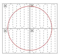
Figure 5. Area decomposed into four subareas by using the back-and-forth pattern.
