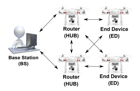
Figure 11. ZigBee devices in a scenario FANET test with mesh configuration.
