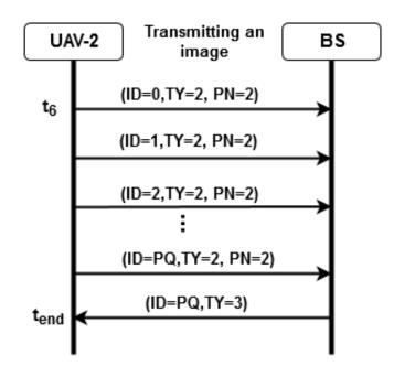
Figure 10. Message flow for transmitting an image.
