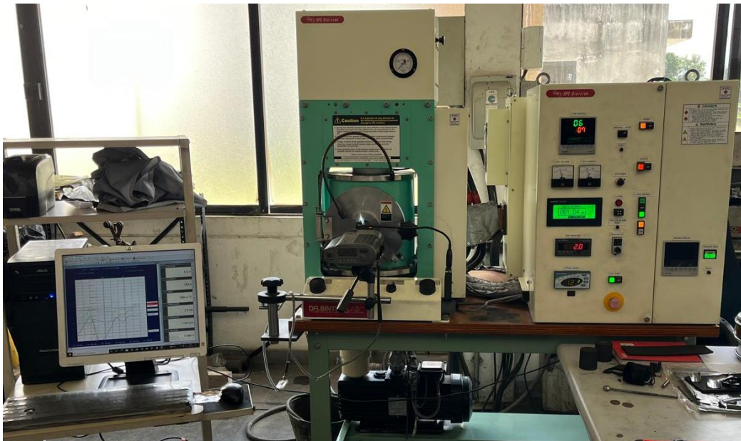
Figura 14. Spark Plasma Sintering (SPS).
