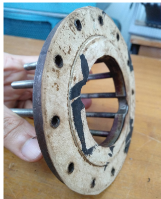
Figure 4.3: Prototype PIG 1. Gasket sheets were installed on the flanges of the PIG to improve sealing.
