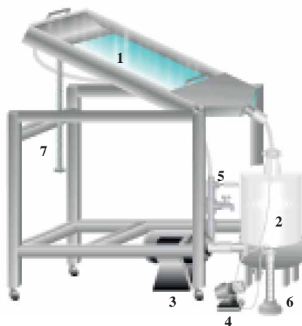
Figure 1. The photochemical system: (1) falling-film solar reactor, (2) stirred tank, (3) centrifuge pump 0.5 CV, (4) peristaltic pump, (5) system of sampling, (6) hydrogen peroxide vessel and (7) regulator screw of slope.
