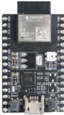
Figura 3 – DevKit Modelo ESP32-C3-DevKitC-02.
