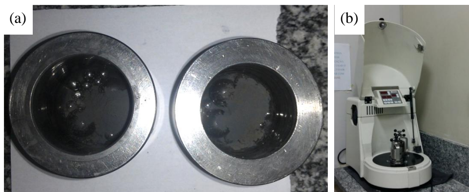
Figure 3.14 Prepared vessel (without cyclohexane) for high energy (a) and Fritsch, Pulverisette 7 milling machine (b).
