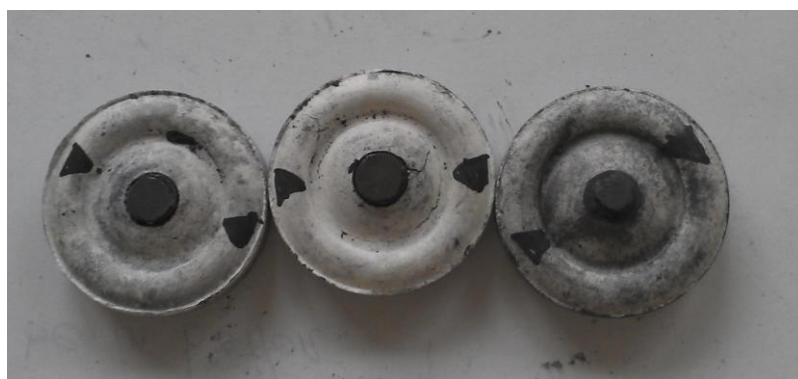
Figure 3.16 Prepared capsule for sintering with mark to show top diamond layer.
