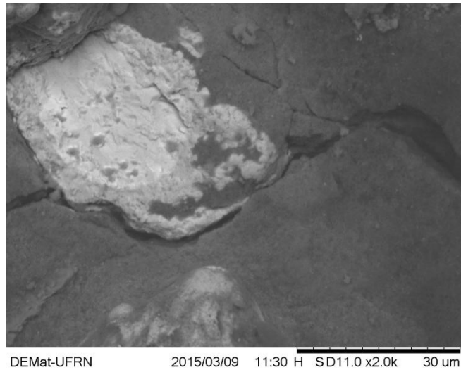
Figure 4.5 Separation of particle and diamond matrix by crack propagation.
