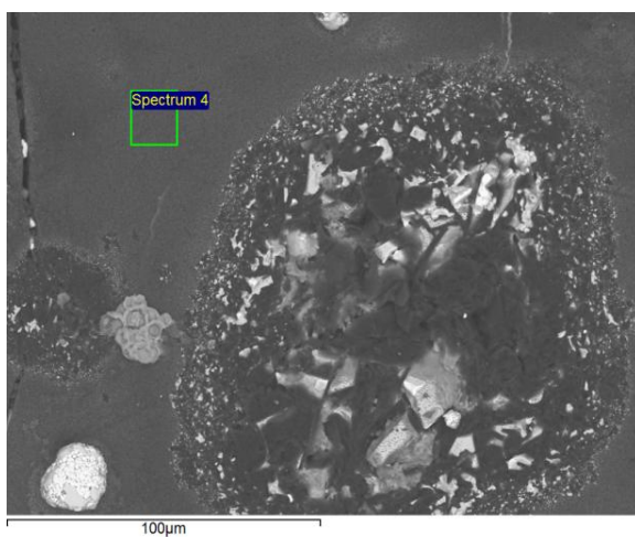
Figure 4.7 Chemical analysis by EDS at an area near Iron particle.
