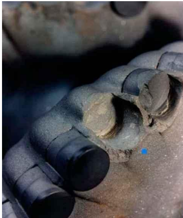
Figure 2.20 A failure in PDC. Diamond layer separated from hardmetal substrate.
