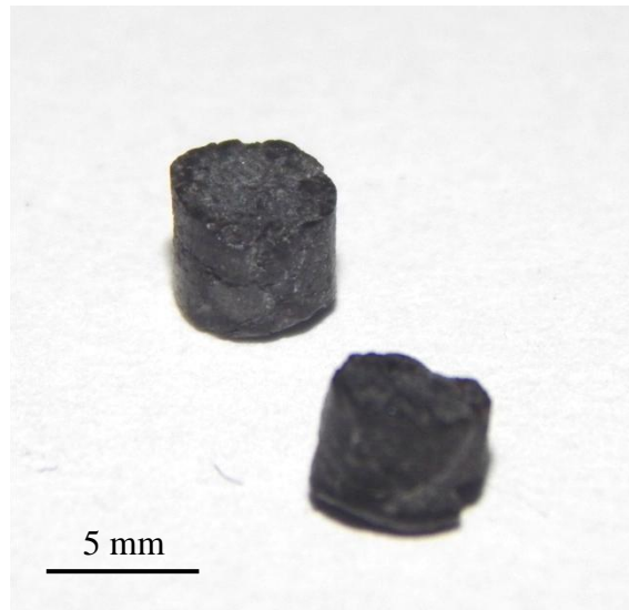
Figure 4.2 Broken sample A 1 sintered at 1600 °C/5.5 GPa/ 3min.
