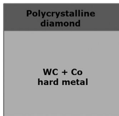
Figure 2.14 Geometry of a typical PDC cutting tool used in oil & gas drilling.
