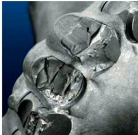
Figure 2.22 A failure in PDC. Fracture inside diamond layer and in hardmetal substrate.
